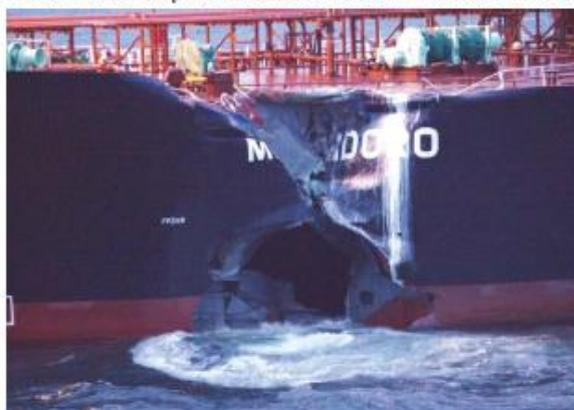
Figure 3 Ship to ship collision damage.
