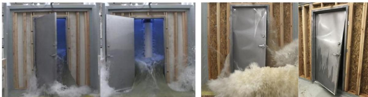
Figure 7-16 Tests on a steel door, with outward pressure (left) and inward pressure (right), photos adopted from Wells et al. (2019)
