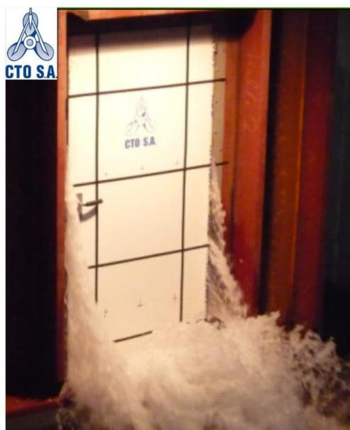
Figure 7-13 Hinged A-class fire door under 12 kPa water pressure; notable leakage, photo adopted from Jakubowski and Bieniek (2010)
