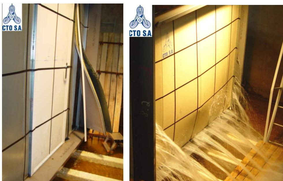
Figure 7-15 B-class fire rated structures in FLOODSTAND tests, damage to wall around a closed door (left) and significant leaking of a wall (right), photos adopted from Jakubowski and Bieniek (2010)
