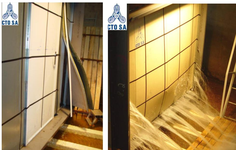
*Figure 4-8 B-class fire rated structures in FLOODSTAND tests, damage to wall around a closed door (left) and significant leaking of a wall (right), photos adopted from Jakubowski and Bieniek (2010)*
