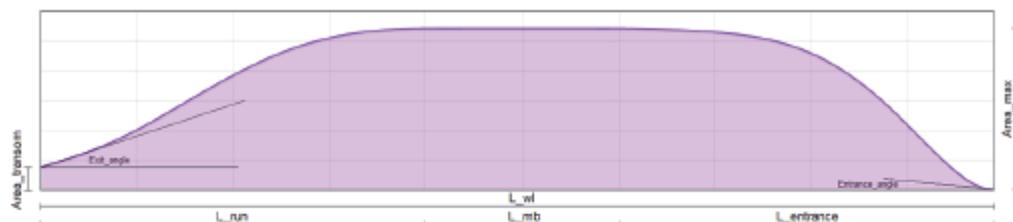
**Figure 4** Sectional area curve of a ship.
