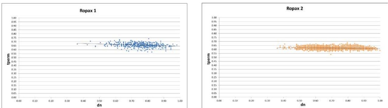
Figure 52 Actual global tanks permeability vs Normalized Draught (ropax ships 1 - 2)
