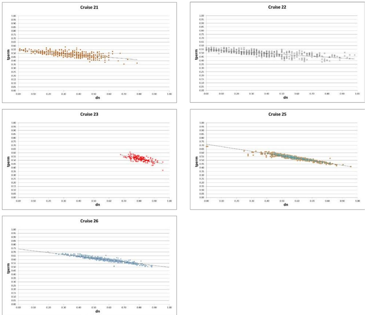
**Figure 43 Actual global tanks permeability vs Normalized Draught (cruise ships 21 – 26)**
