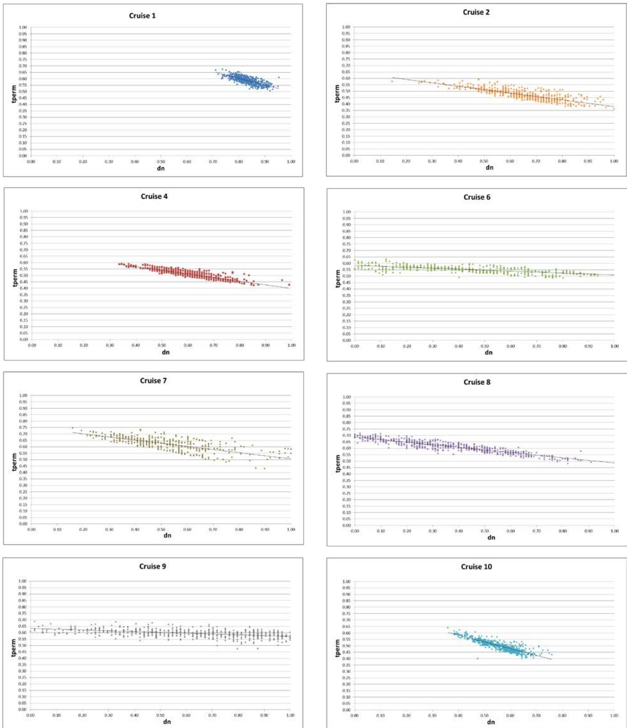
Figure 41 Actual global tanks permeability vs Normalized Draught (cruise ships 1 – 10)
