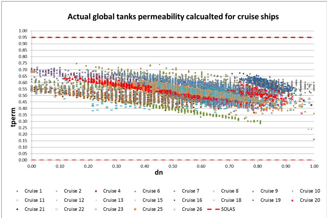
Figure 44 Actual global tanks permeability vs Normalized Draught (all cruise ships)
