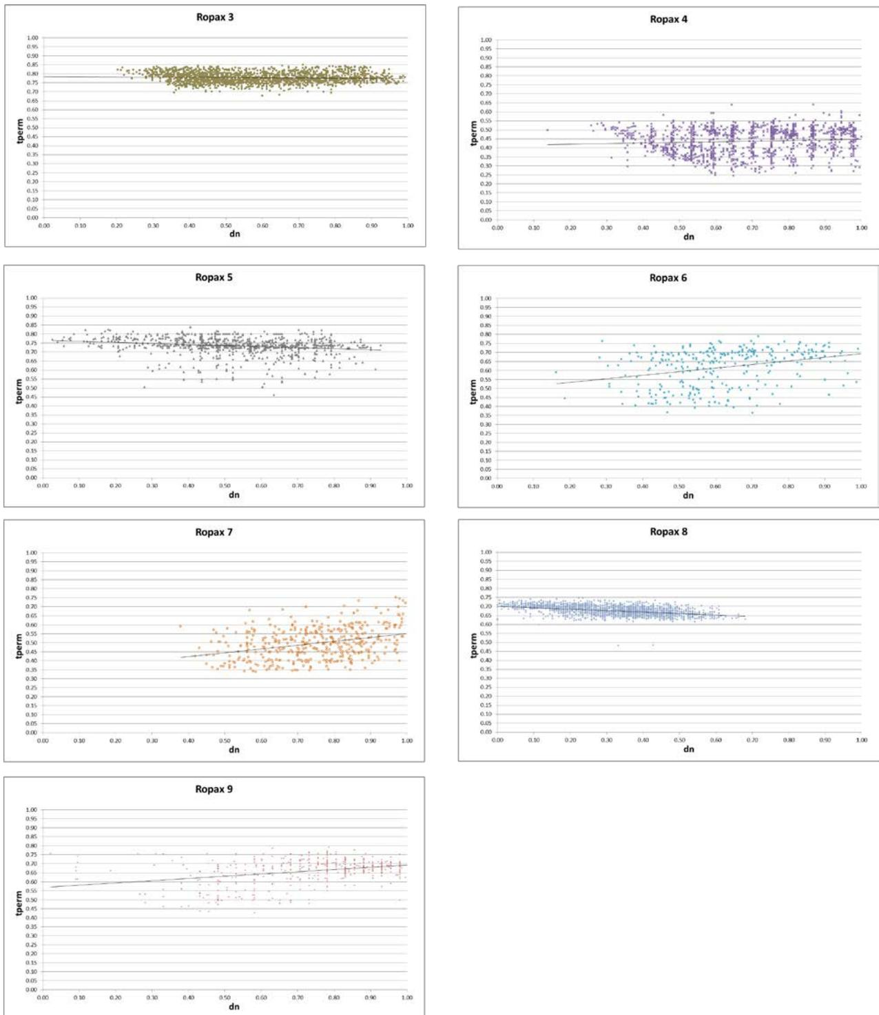
Figure 53 Actual global tanks permeability vs Normalized Draught (ropax ships 3 - 9)
