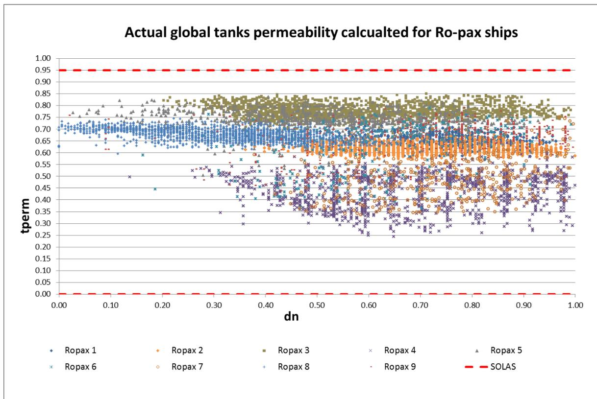
Figure 54 Actual global tanks permeability vs Normalized Draught (all ropax ships)
