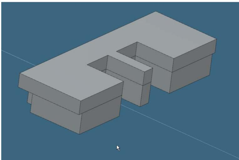
**Figure 18 Reference 3D-shape of auxiliary engine room #1**
