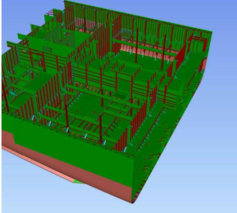
**Figure 11 Steel structure of Main Engine Room #2**
