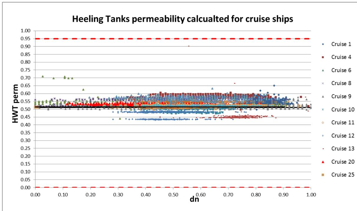
Figure 46 Actual Heeling Tanks permeability (HWTperm) vs Normalized draught (dn)
