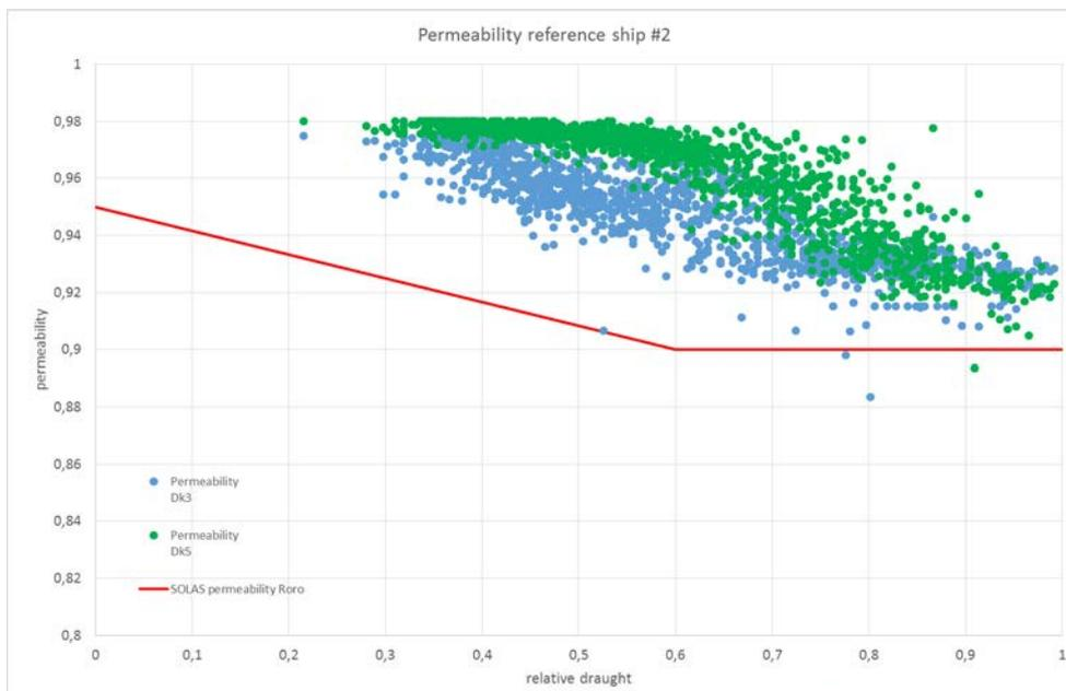
Figure 37 Permeability of cargo holds ship #2
