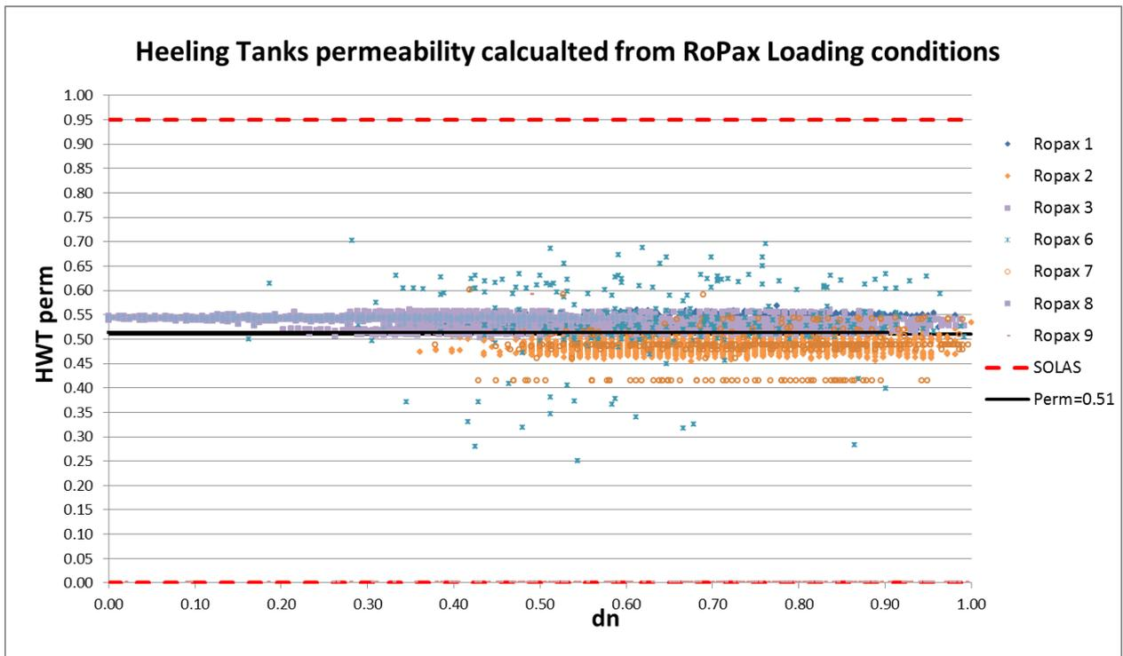
Figure 55 Actual global tanks permeability for Heeling tanks (ropax ships)
