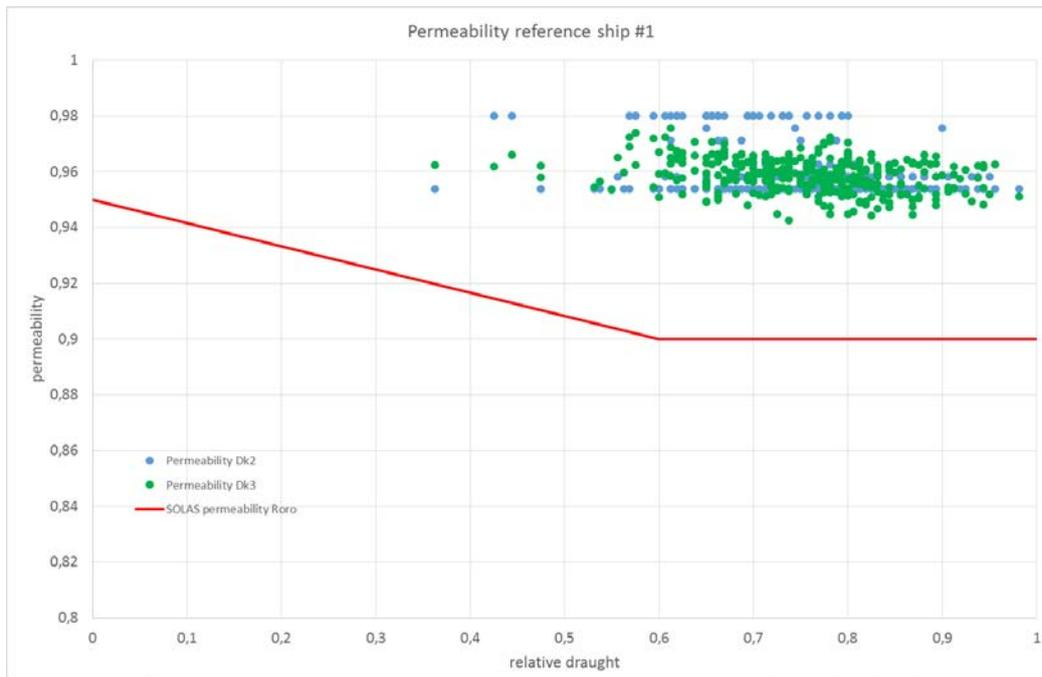
Figure 36 Permeability cargo hold ship #1
