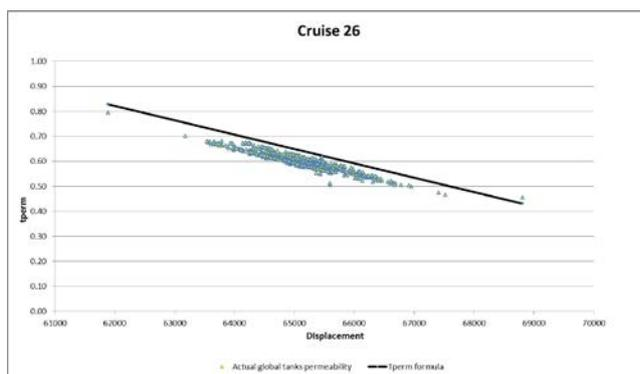
**Figure 49 Actual global tanks permeability vs Displacement (cruise ship 26)**
