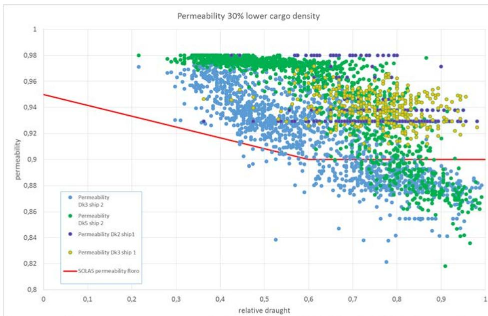
**Figure 39 permeability of cargo holds with 30% lower density**
