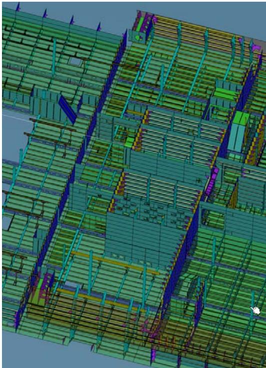
**Figure 20 Steel structure of auxiliary engine room #1**
