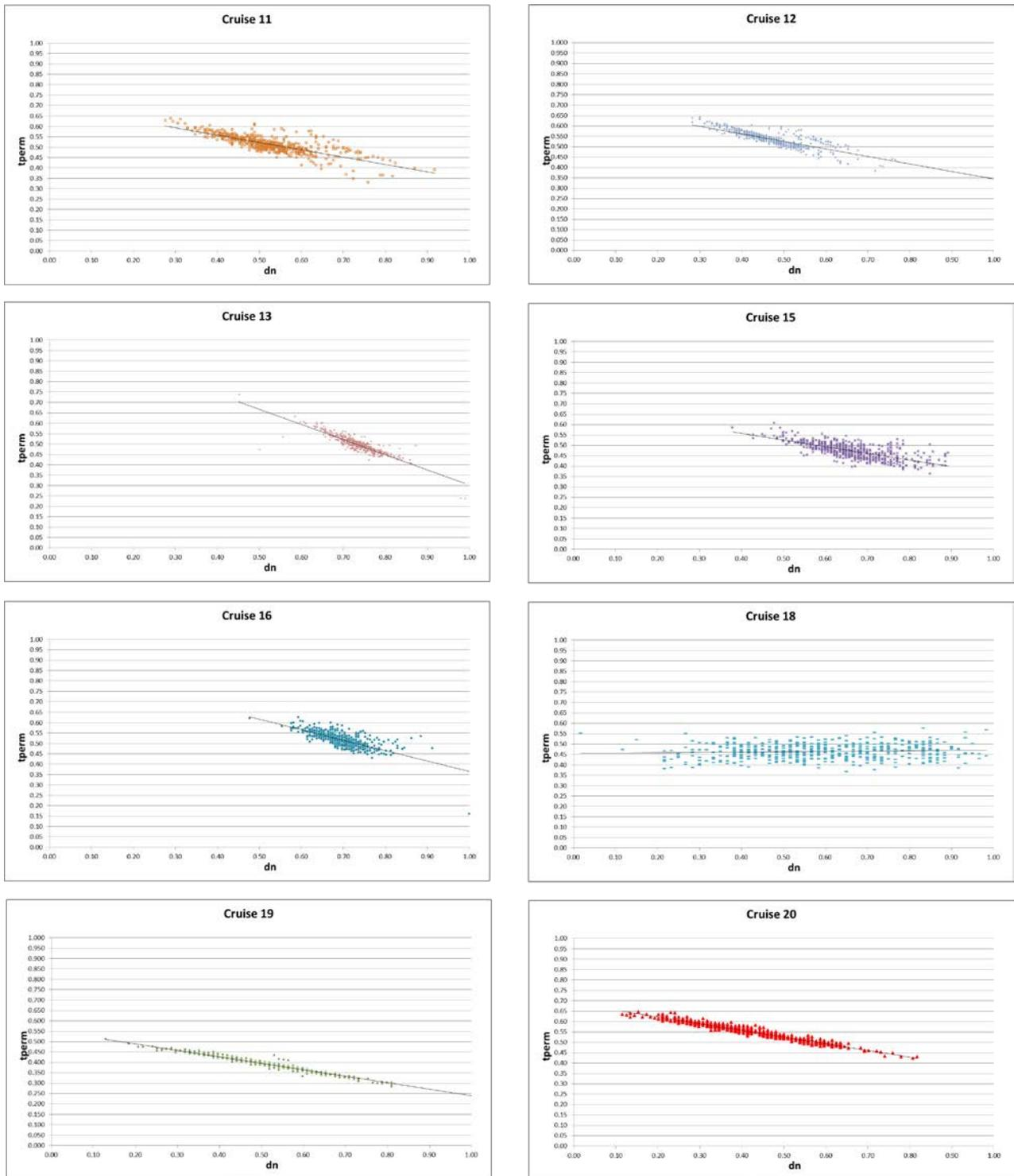
Figure 42 Actual global tanks permeability vs Normalized Draught (cruise ships 11 – 20)
