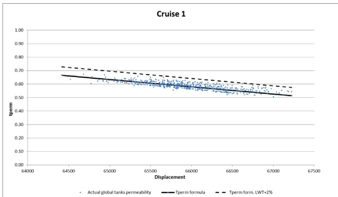
Figure 50 Tanks permeability calculated with Mathematical formula and 2% Lightweight margin
