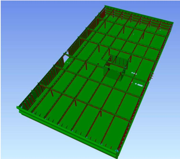
Figure 29 Cabin area #2 steel structure
