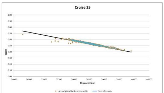
Figure 48 Actual global tanks permeability vs Displacement (cruise ships 12 – 25)
