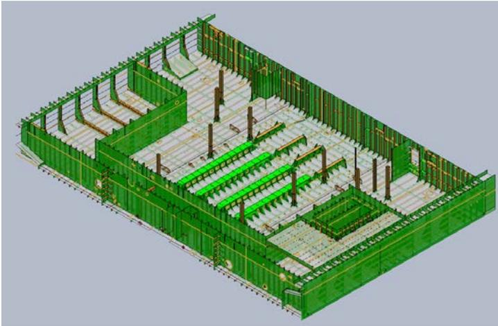
**Figure 15 Steel structure of MER #3**
