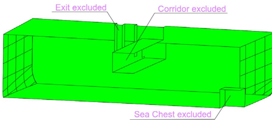
Figure 8 3D-shape of Main Engine Room #2 (aft view)
