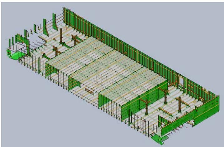
**Figure 24 Steel structure of auxiliary engine room #2**
